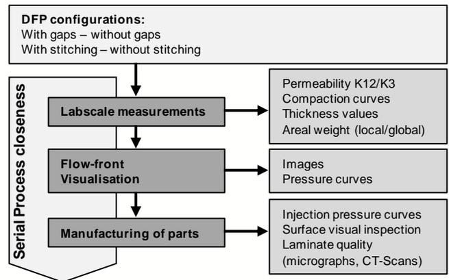
Figure 2: Methodology and evaluation parameters
